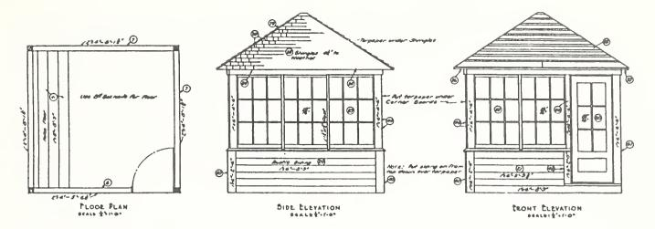
Figure 60. Patrol shelter or tower cupola, 1932, Northern District No. 1. Shown in plan as well as in side and front elevations, this eight foot square L-6 type structure could be used either on the ground or with T-1 and T-2 towers.
